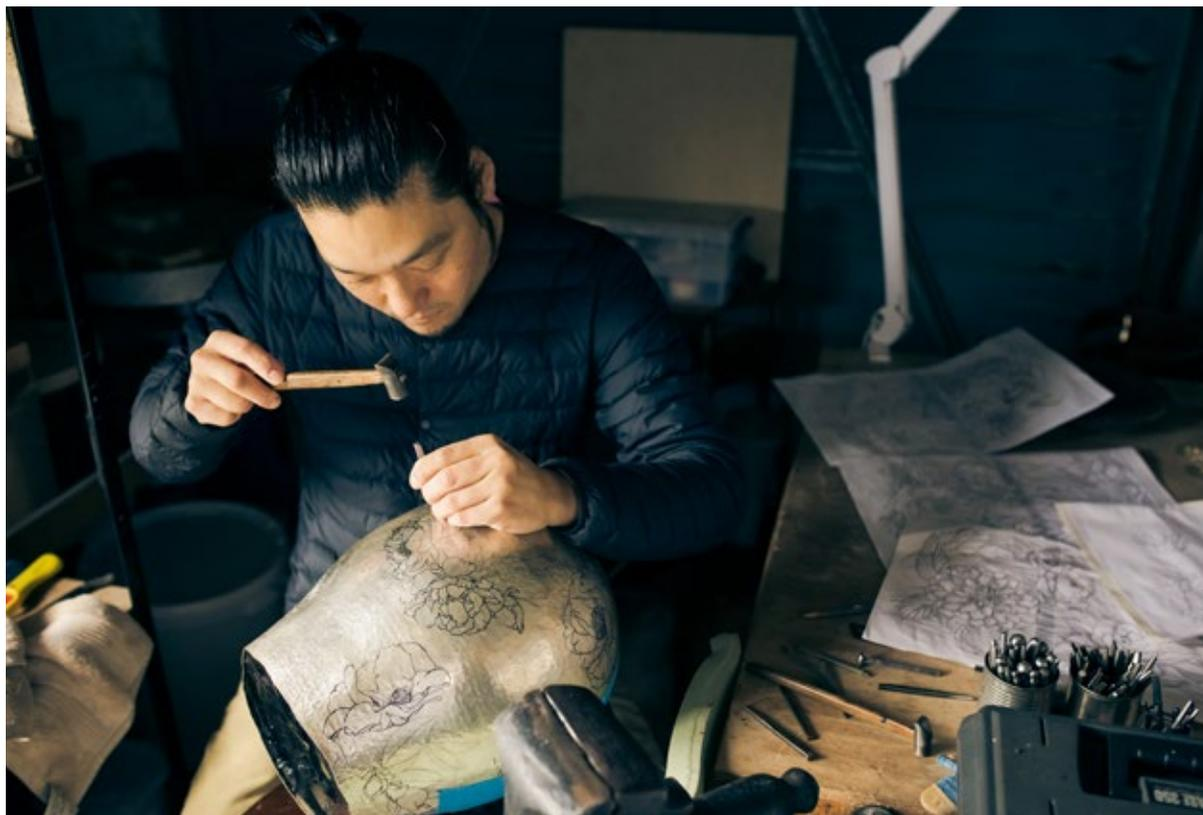
pitch inside a piece with a heat gun – like a strong hairdryer – when he is chasing to make the silver easier to work with.
