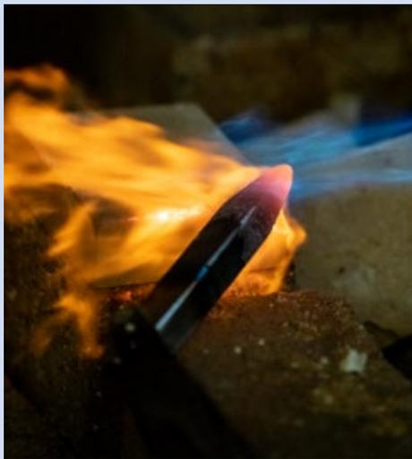
5. The punch is heat-treated to harden and temper it.
